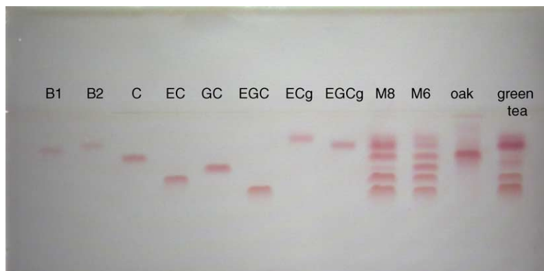
Fig. 6. The separation of flavan-3-ols test mixtures (M6 and M8), oak and tea extracts on HPTLC plates developed using 1-propanol–water (20:80, v/v) in horizontal developing chamber (sandwich configuration).
